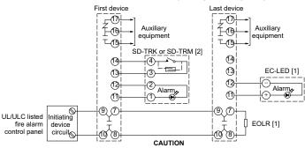
Do not use looped wires under terminals 9 and 7, or 10 and 8. Break wire run to provide supervision of connections.
